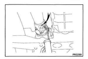
B. APPLY MP GREASE TO GREASE FITTING
