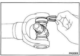
(f) Install two snap rings of equal thickness which will allow 0 - 0.05 mm (0 - 0.0020 in.) axial play.
