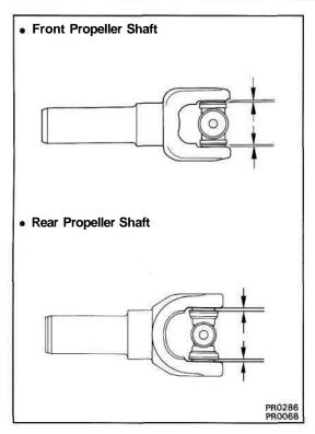
(e) Using SST, adjust both bearings so that the snap ring grooves are at maximum and equal widths.
