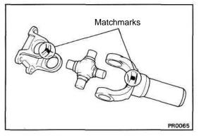
(b) Align the matchmarks on the yoke and flange.
