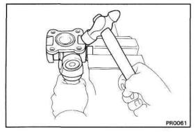
(e) Clamp the bearing outer race in a vise and tap off the flange with a hammer.
