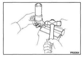
(h) Clamp the outer bearing race in a vise and tap off the yoke with a hammer.
